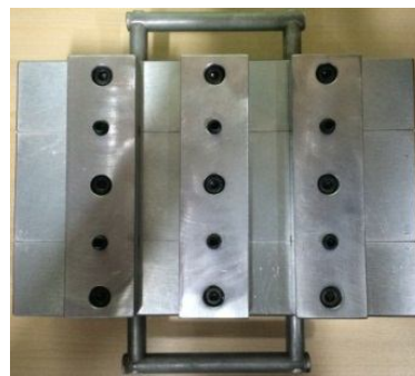
图 2 胶结成型装置 Fig.2 Devices for bonded specimen preparation
